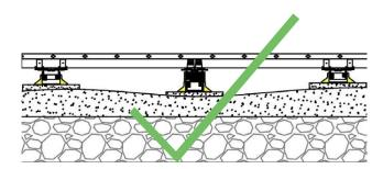
NewTechWood products can be stored on pedestals or jacks if the surface is uneven, as shown above. Consult with the pedestal or jack manufacturer before using the product to ensure its compatibility with NewTechWood's products.
