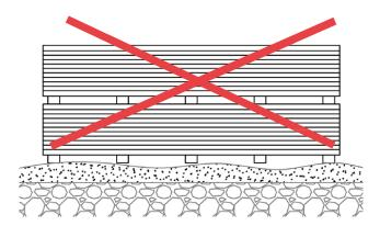
NewTechWood products stored on an uneven surface will make the products prone to warping and distortion.
