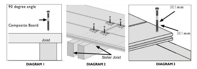
Use screws designated for use with composite decking material. Always test the screws on a scrap piece of board to ensure the screws do not cause the surface of the decking to mushroom or bulge around the head of the screw. If it does cause this issue, change to a different brand of screw.
