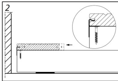
Take the grooved board and push it into the starting clips.
