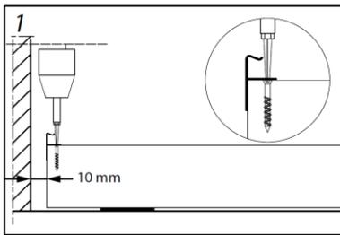
Install the K37/MG3 starting clips – centred at the edge of each.
