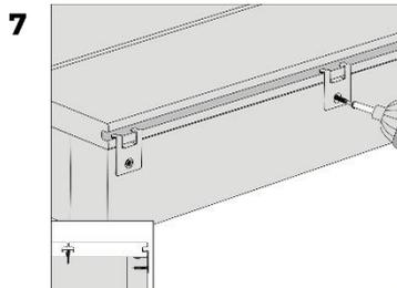
For the final board use the start/end fasteners and screw the fastener in from the side to fix the last board in place.
