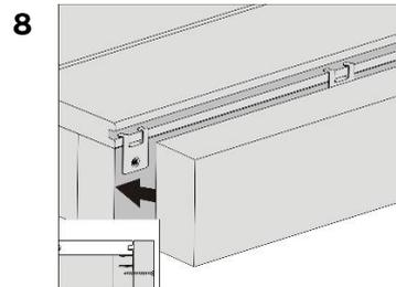
Finally, install the fascia using two composite screws – every 400mm centre to centre. **Fascia boards always need to be pre-drilled and countersunk before they can be face fixed.**
