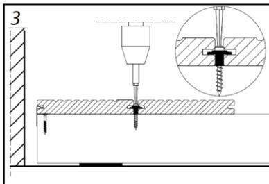
Insert the Cobra T-Clip into the grooved edge of the deck board. Slide the second board into the hidden fastener. Screw down the hidden fastener.
