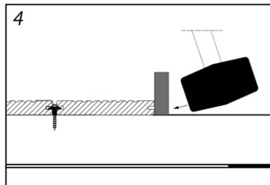
Tighten the second board with a rubber mallet to ensure a consistent gap of 6mm max between the two boards.
